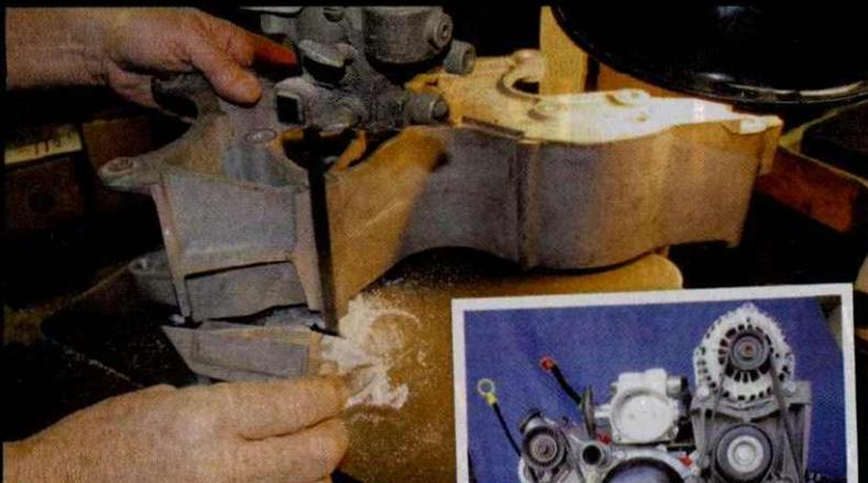
We trimmed the stock truck bracket using a bandsaw. You could use a hacksaw or a cut-off wheel, but the bandsaw leaves a much cleaner cut.
