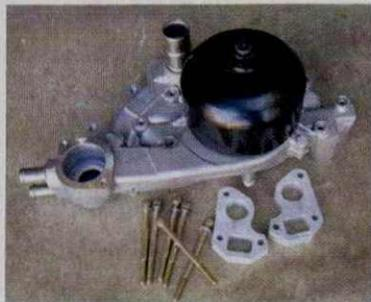
The truck's water-pump outlet is also an obstruction, so LS Brackets offers this water-pump spacer kit complete with new gaskets and longer Allen bolts. The spacers relocate the F-car water pump to align the pulley with the deeper truck orientation. This also requires an F-car tensioner. We obtained both the water pump and tensioner from RockAuto and saved more than \$75 compared to our local auto parts chain store price, even with the shipping cost.
